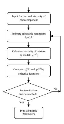
Figure 1. Flow chart for the calculation procedure based on GA method.
