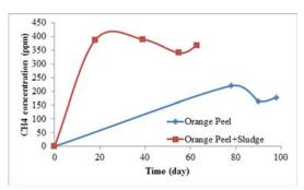
Figure 4-c. Methane gas concentration in the biogas produced from orange peels with and without sludge  $(T = 35^{\circ}C)$ .
