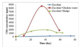
**Figure 4-a**. Methane gas concentration in the biogas produced from zucchini in the presence of sludge, and chicken dung as an inoculum 35°C.
