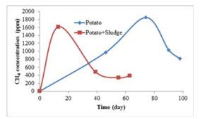
**Figure 4-b.** Methane gas concentration in the biogas produced from potatoes with and without sludge (T=35°C).
