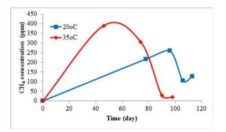
Figure 3c. Methane concentrations in the biogas produced from tomatoes at 20°C and 35°C.
