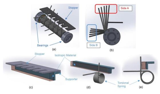
**Figure 5.** (a) An isometric material and (b) a side views for the structure of the passive toe joint part for the biomechanical leg. (c) A supporter for the isotropic material is attached below the stopper, (d) the stopped is hidden and one of the five springs is shown in front of the isotropic material, and (e) a side view for the structure.
