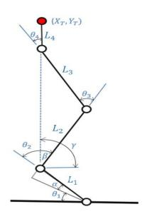
**Figure 8**. Biomechanical leg model with a fixed toe joint position to perform the first stage of the stance motion.
