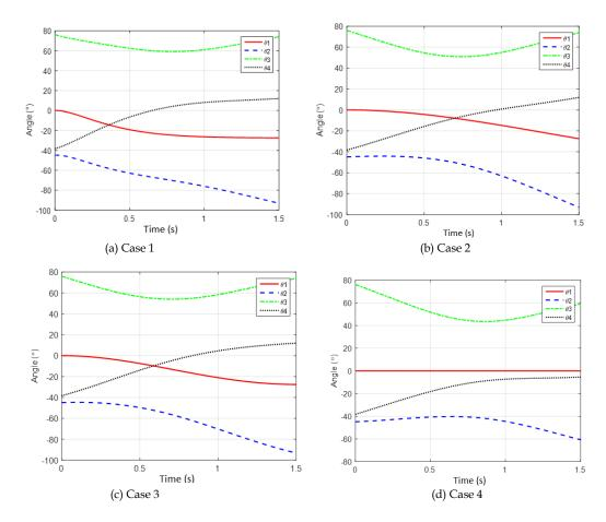
**Figure 9**. The calculated changes in the joints angles ( $\theta_2$ ,  $\theta_3$ , and  $\theta_4$ ) for a given torso movement, with different trajectories (different cases) of toe joint ( $\theta_1$ ).
