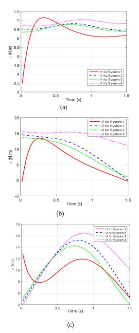
**Figure 10**. The calculated torques in the joints: (a) Toe, (b) Ankle, and (c) Knee for a given torso movement, with different trajectories (different cases) of toe joint ( $\theta_1$ ).
