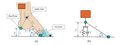
**Figure 6**. (a) A sketch of a human foot with mass-spring damper system model, for the toe joint, which uses torsion spring and damper. (b) Equivalent mass-spring damper system model that uses linear spring and damper.
