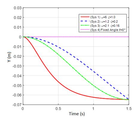
**Figure 7**. The vertical displacements of the heel point, in the biomechanical foot, caused by the rotational movement of the toe joint by 30<sup>o</sup> for case 1, case 2, case 3, and case 4.
