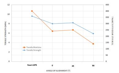
Figure 3. Tensile strength (left) and Tensile Modulus (right) of the tested bio-composites sheets.
