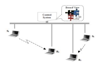
**Figure 5**. Network model and topology as used in the simulation. The nodes disseminate the estimated link gain to get broader view and perform joint optimization.
