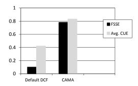
**Figure 12**. Performance evaluation of 50 nodes in a random topology in terms of fairness FSSE and average channel usage efficiency CUE, using the default DCF and CAMA mechanism.
