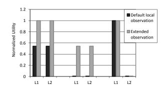
**Figure 3.** Normalized utility for the scenarios in Fig. 2, in terms of MAC's layer good put with default channel assessment at the senders and extended assessment to the intended receiver.
