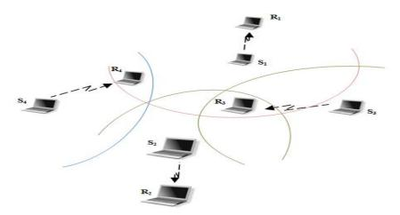
**Figure 8**. Four sender-receiver pairs distributed in three-dimensional distribution in 100x100x100m3 indoor environments with disparity in link quality.
