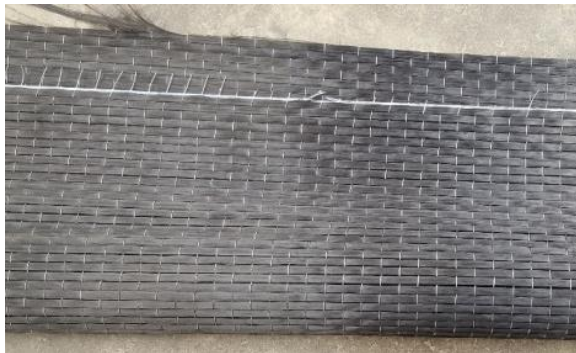
Figure 2. Unidirectional CFRP sheets used in this study.
