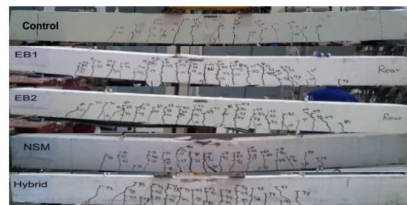
Figure 10. Tested beams after failure.
