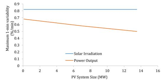
Figure 5. Maximum 1-min variability of a 13.2-MW PV plant on a highly variable day (Mills 2010).
