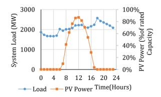
Figure 2. Manah site solar PV system output (clear sky) and recorded MIS system load data on 1 January 2015.
