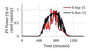
Figure 3. Manah site 1-minute PV power output data for 2 days in 2015 (passing clouds).
