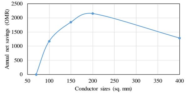
**Figure 6.** Annual net savings variation for different sizes of overhead conductors for annual peak load current 120 A, 0.5 load factor, where the optimal conductor size is 200 sq. mm.
