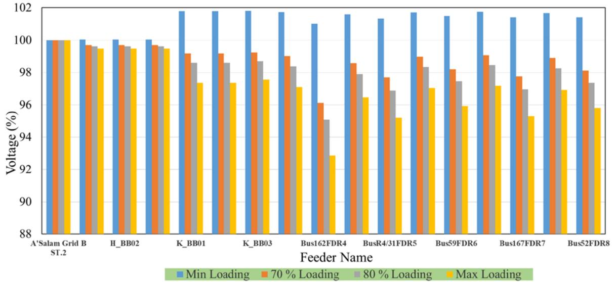
Figure 3. Voltage profiles for the selected buses at different loading conditions.
