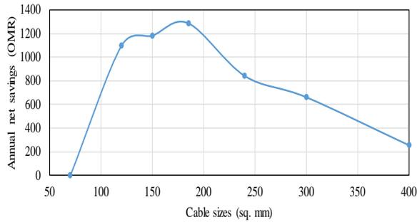
**Figure 5.** Annual net savings variation for different sizes of cables for annual peak load current 120 A, 0.5 load factor, where the optimal size is 185 sq. mm.
