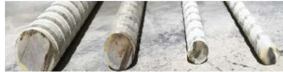
(a) Grooved GFRP Bars (G1).
