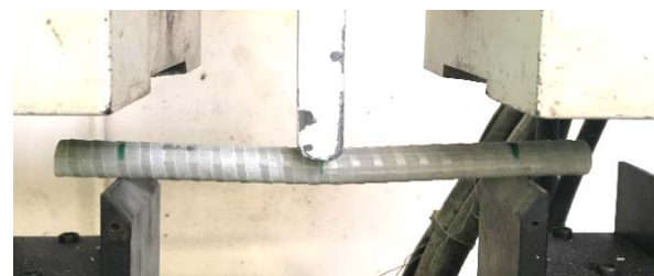
Figure 2. FRP specimen during flexure testing.
