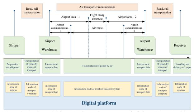
**Figure 10**. The scheme of information interaction among supply chain participants including air transport based on the digital platform
