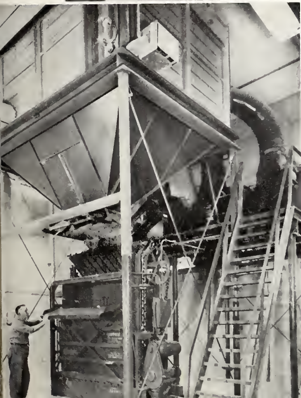
Vacuum-sweep equipment draws paper trim and waste into huge baler, at left.
