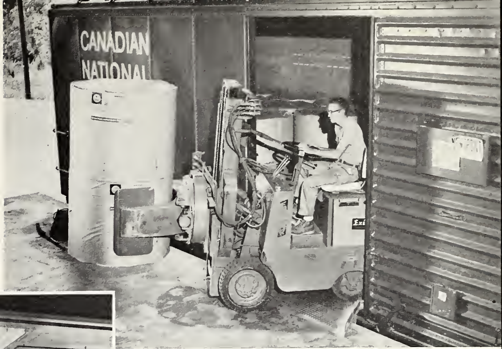
Newsprint and magazine paper are unloaded from freight cars inside OSV's building. Clamp-lift trucks handle the rolls which weigh up to 2,000 pounds.
