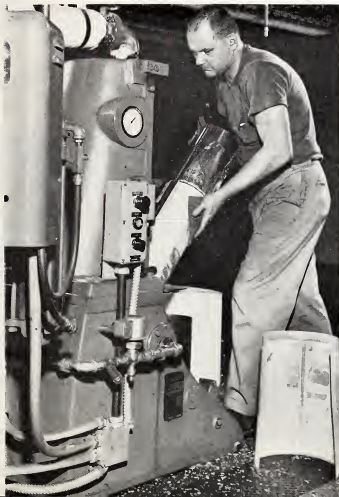
At left, Thomas Kindler removes stereotype plate from casting box. Below, Gene Rudicel operates Fairchild Scan-a-Sizer for plastic engravings.
